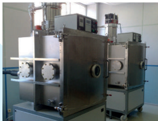
VACUUM ELECTRON BEAM 3D PRINTER. POWDER SINTERING. BUILD-UP AREA – 300 MM IN DIAMETER, HEIGHT 400 MM
